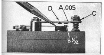
The cushion spring is the final static adjustment. Here, with the lower contact held against the core, there needs to be about 0.005" between the cushion spring and the upper vibrator, shown at point A. This is achieved by slightly bending the upper vibrator which can be done by gently tapping on point D.
