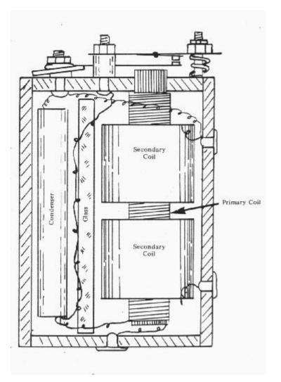
The amount of energy stored in the iron core is determined by how much current flows through the low voltage primary winding, and for how long. These factors are largely determined by the points adjustment and supply voltage.
