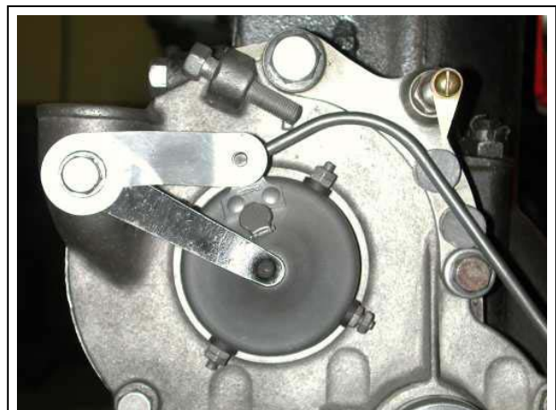
Figure 3—Timer Mounted on Engine Using Original Ford Adjusting Gauge Photo Courtesy of Steve Coniff
