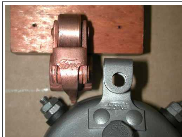
Figure 2—Ford Script on Timer Case and Roller. Photo Courtesy of Steve Coniff
