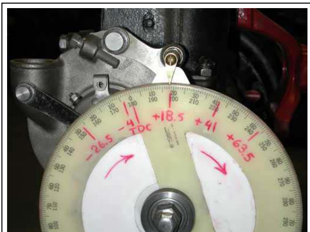
Figure 6—Degree Wheel Mounted on Crankshaft, with Pointer Photo Courtesy of Steve Coniff
