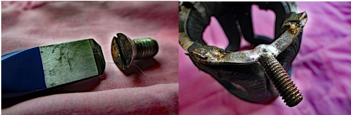
I had been given a set of (Aldi) metal chisels including a range of standard cold chisels and selecting one that had the same width as the top of the screw I ground off the chisel point and squared the end so it was a neat fit in the screw slot with no side draft and then ground the 2 ends of this blade so it matched the slope of the countersink face of the head of the screw.
