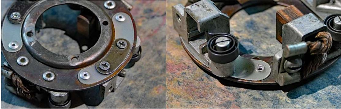
To refit the brush holder plate to the end cap I made a hollow point punch using a hi-tensile bolt drilling and the grinding the hole in the end to produce a reasonable shaped head on the brass rivets.
