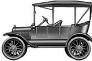
Touring - Open Car - folding top, no side windows, front and rear seats.
