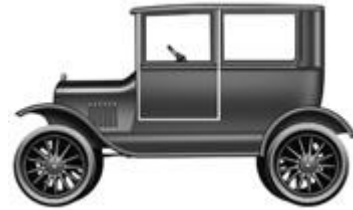
Tudor Sedan - Closed Car - two doors, enclosed interior with front and rear seats, side glass windows.
