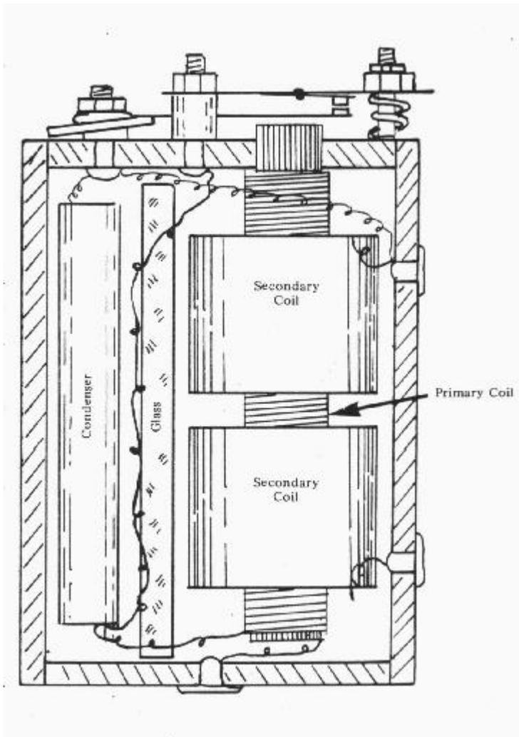
The amount of energy stored in the iron core is determined by how much current flows through the low voltage primary winding, and for how long. These factors are largely determined by the points adjustment and supply voltage.
