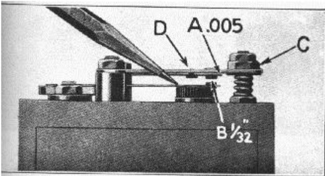
The cushion spring is the final static adjustment. Here, with the lower contact held against the core, there needs to be about 0.005" between the cushion spring and the upper vibrator, shown at point A. This is achieved by slightly bending the upper vibrator which can be done by gently tapping on point D.
